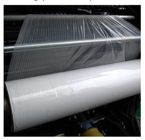
A AGRONIC MidiFix II can optionally be equipped with a film binding system. When this is present on the machine, it is also still possible to use net. Changing film or net is just changing a setting in the control system.
