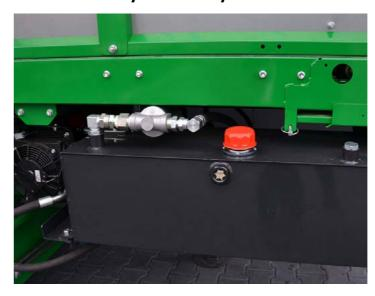
AGRONIC MultiBalers are standard equipped with their own hydraulic system based on two oil pumps. An oil cooling system is also included.
