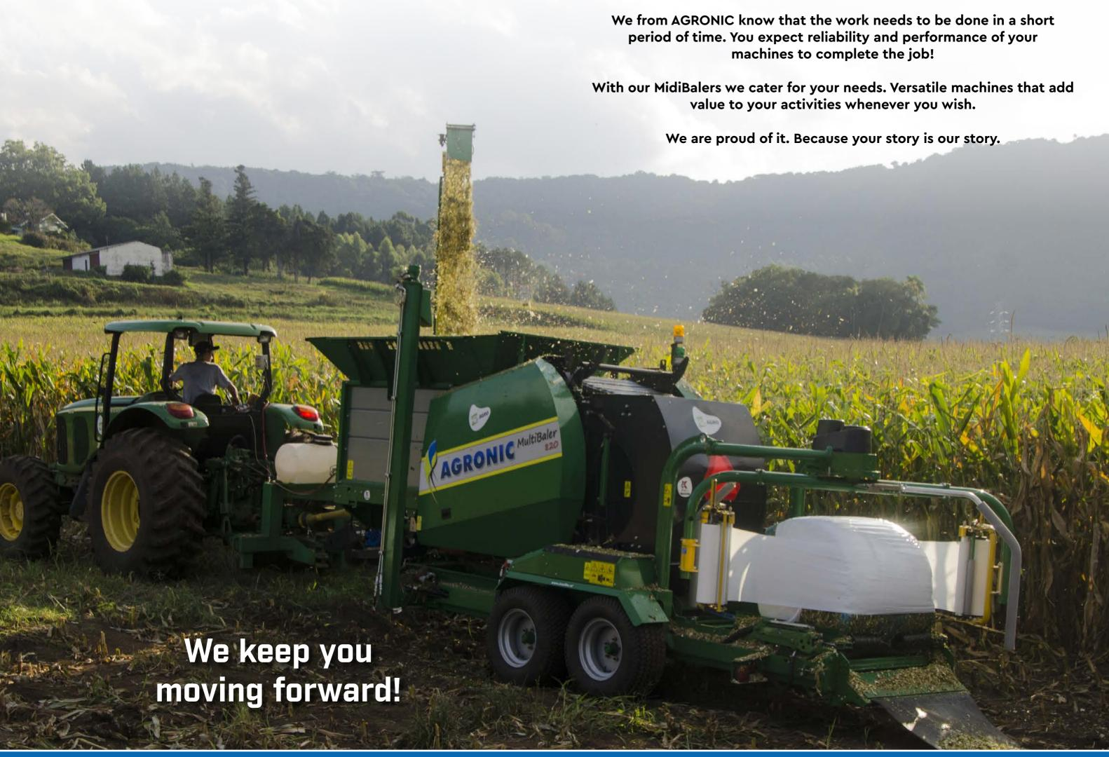
The AGRONIC MultiBaler 820 is a compact machine for processing short crops & materials into 'midi' sized round bales. Midibales are ideal for users with a low feed rate and are very manageable due to their size and corresponding weight.
