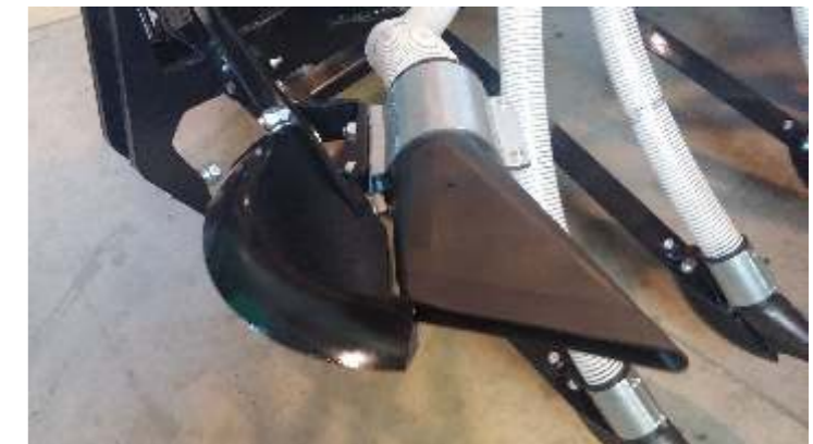
The frame of the spreading ramp can turn and tilt independent of the slurry tank.
