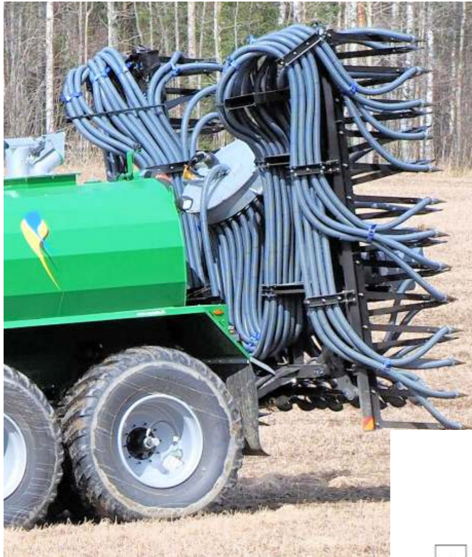
The transport position is compact, wing folding is automatic
