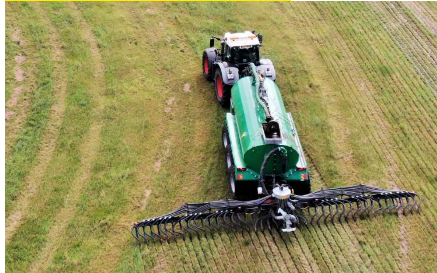
The frame of the spreading ramp can turn and tilt independent of the slurry tank.
