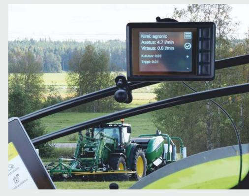
Optionally available is this display device. Here the application system has a trip master function, a designated counter with 8 memory locations, as well as programmable transfer pump function, along with the S-Control: in which a fully automated application setting can be created.
