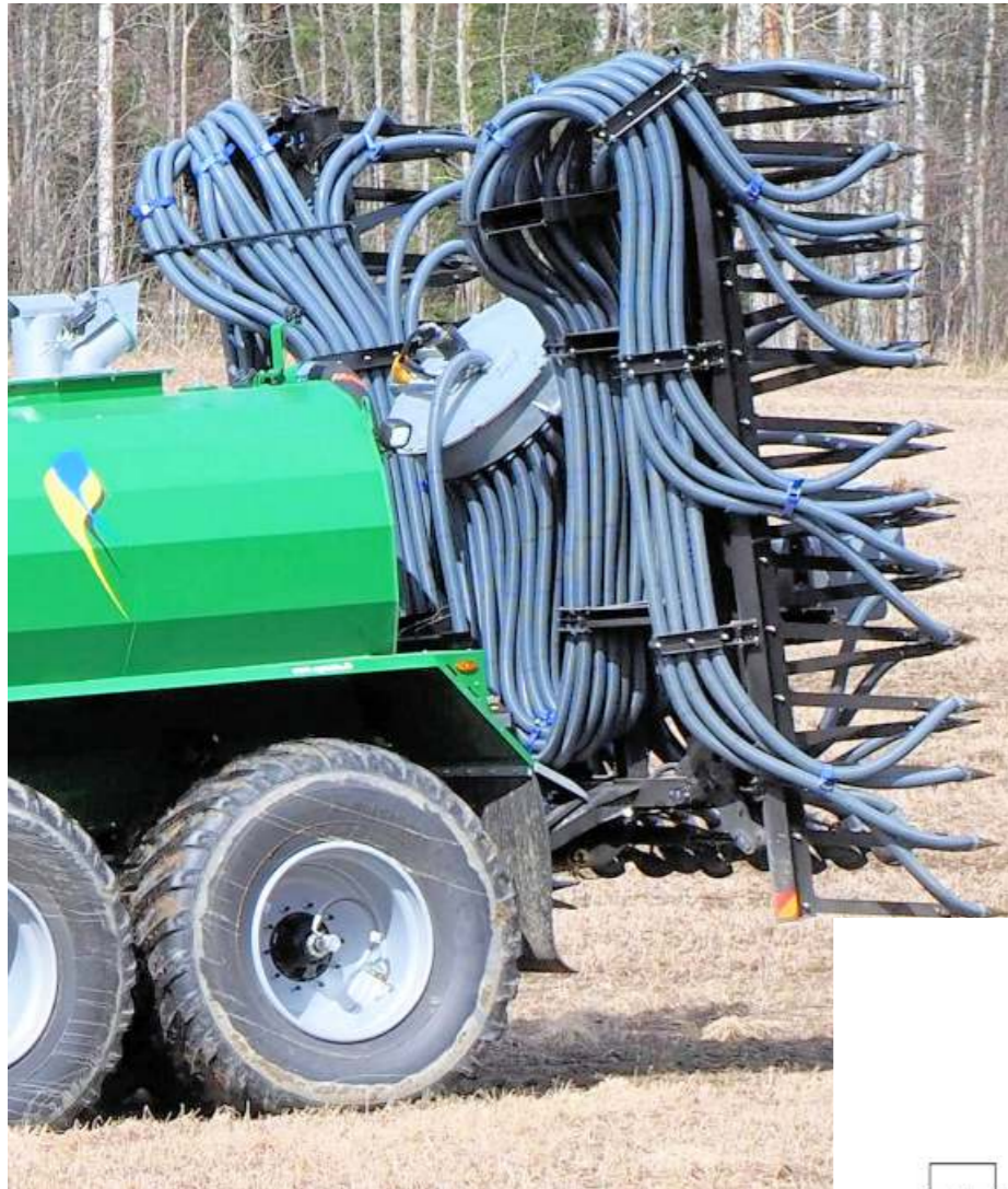
The transport position is compact, wing folding is automate
