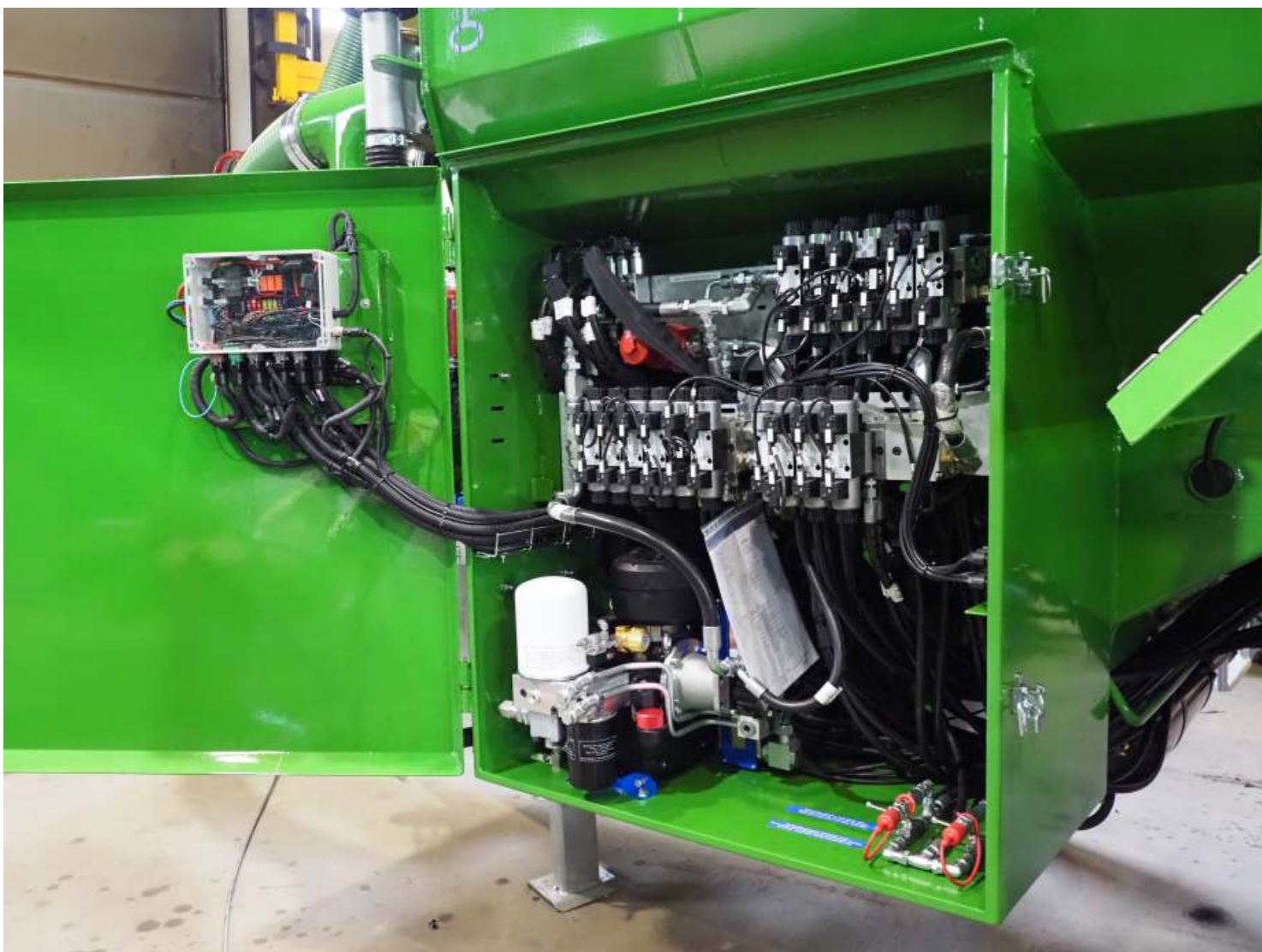
The AIR system is fully integrated into the tanker's control system. Compressor is located in the hydraulic cabin.
