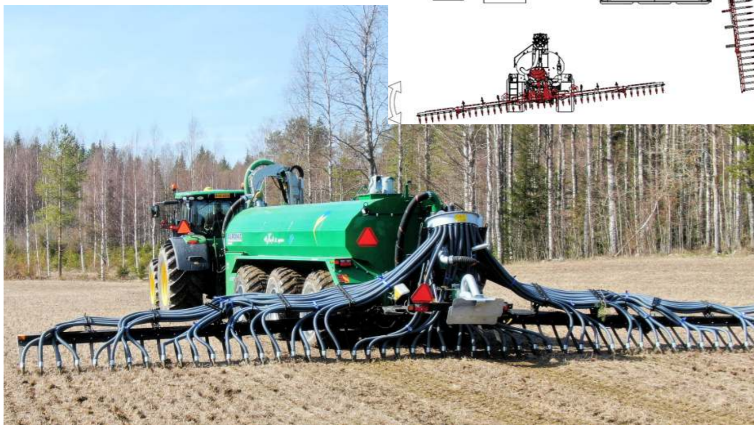
The transport position is compact, wing folding is automate
