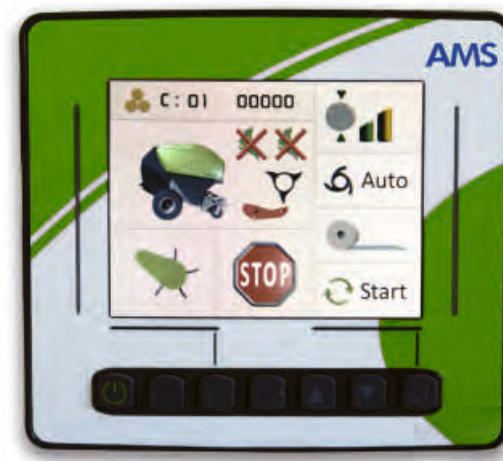
Easy-to-use display for the Agronic AMS. The number of knives selected and raise/lower of the knife cassette Three position bale compression adjustment Completion of the bale is indicated by a colour display and an audible warning. Automatic or manual net binding. Bale counter, bales/hr., total number of bales, and field/customer name can be stored in memory.
