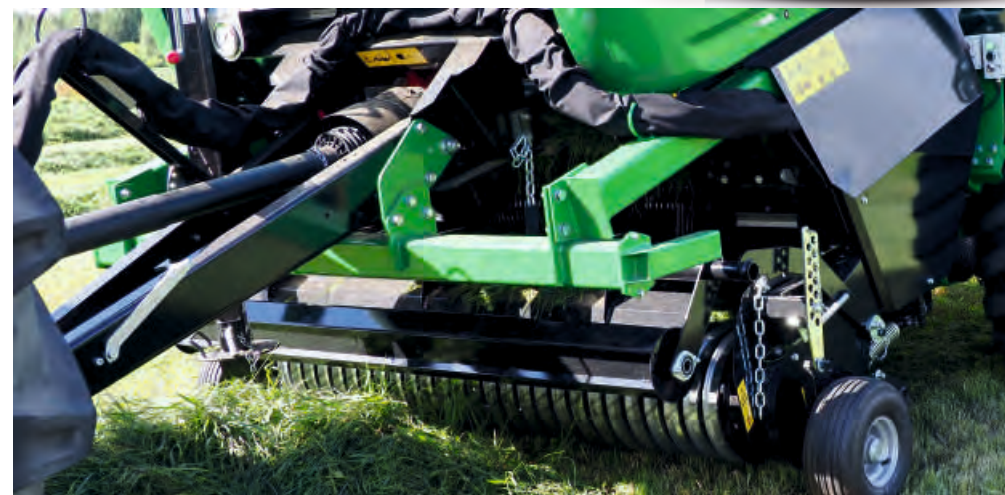
Wide-angle PTO shaft with overload clutch connected to a central gearbox, splits the power to both sides of the baler. On the left side for roller transmission, on the right side for the pick-up and the in-feed roller.
