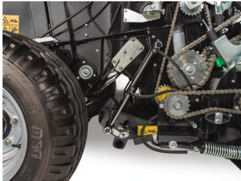
The knife cassette can be lowered electro-hydraulically in the event of a blockage to allow for easy clean-out. Suspended pick-up for optimal ground-contour following. Automatic overload protection.
