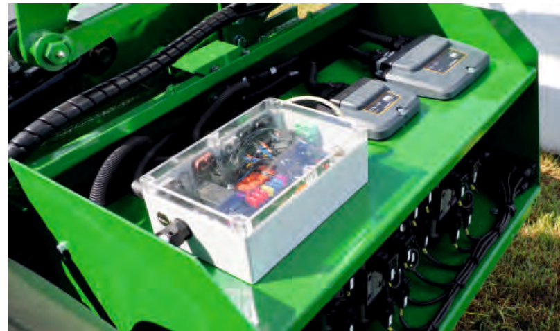
Factory-installed, in-house manufactured, PDH-10 additive application system.
