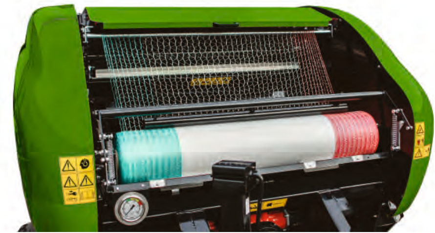
Large and easily accessible compartment for the net, accomodating rolls with widths of 1230 to 1330-mm (4' and 4' 3"). Mechanical net volume indicator and mechanical brake adjustment Reliable design, and easy-to-change the net rolls. Holder for two rolls of net and a low roll loading height.
