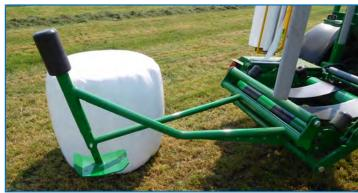
By means of the sidetip the machine automatically unloads the bale on the side. The sides of the wrapped bale have multiple film layers, so damage should be prevented by a hard stubble.
