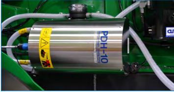
Fully automatic dosing system for adding silage additives during baling. Pump capacity 10 ltr./min.
